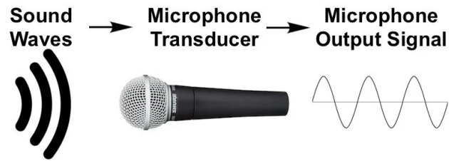
Figure 2.3: Visualisation of how sound waves are converted to a continuous electrical signal. Reproduced from My New Microphone (2019).
